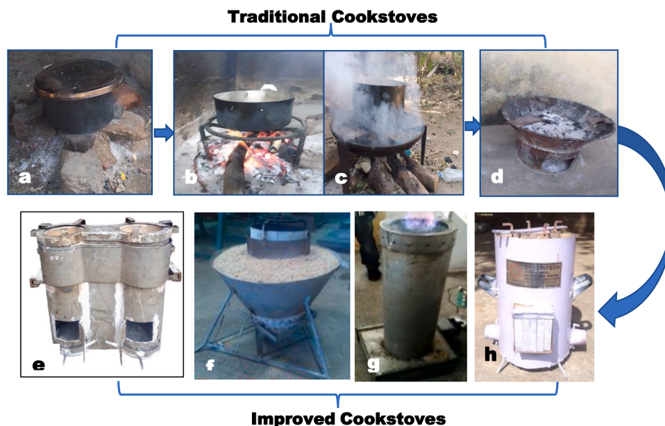
Fig. 1. (a) Three stone open fire, (b and c) metallic open fire, (d) traditional charcoal stove, (e) Natural-draft double burner biomass cookstove [47], (f) husk biomass cookstove [48], (g) Inverted downdraft gasifier cookstove [49], (h) Improved biomass cookstove [50]
