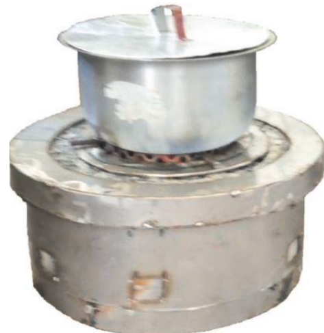
Fig. 5. Granite rock insulated cookstove [70].
