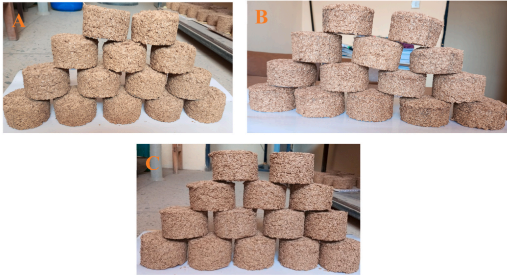
Fig. 2. Briquette samples of (A) locust bean pulp (LBP) binder, (B) sweet potato peel (PPL) binder, and (C) cassava starch (CSS) binder.
