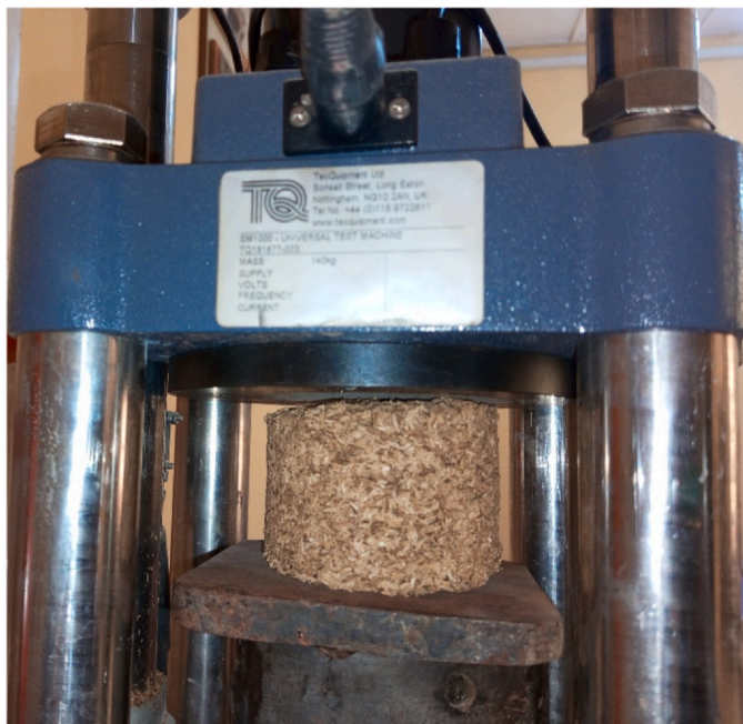
Fig. 3. Determination of compressive strength of a briquette sample using the universal test machine.
