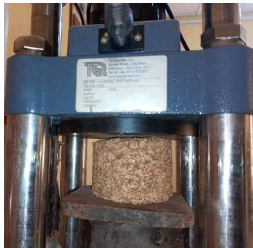
Figure 6.3. Determination of compressive strength of a briquette sample using the universal test machine
