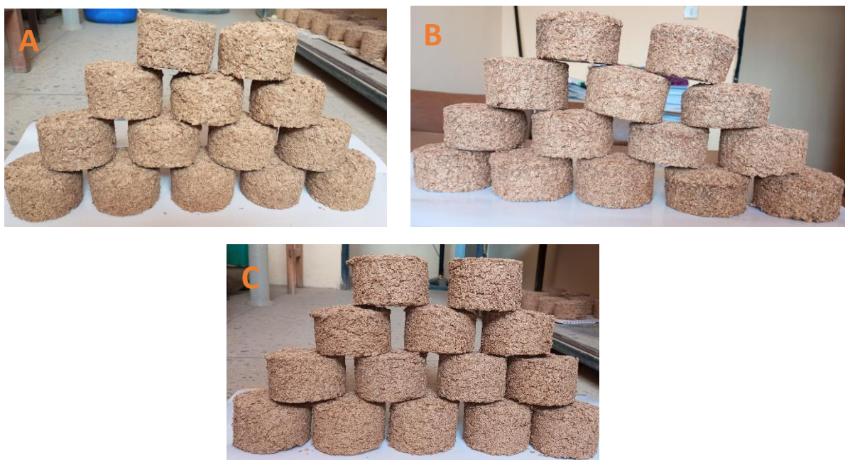
Figure 6.2. Briquettes samples of (a) Locust bean pulp (LBP) binder, (b) Sweet potato peel (PPL) binder, (c) Cassava starch (CSS) binder
