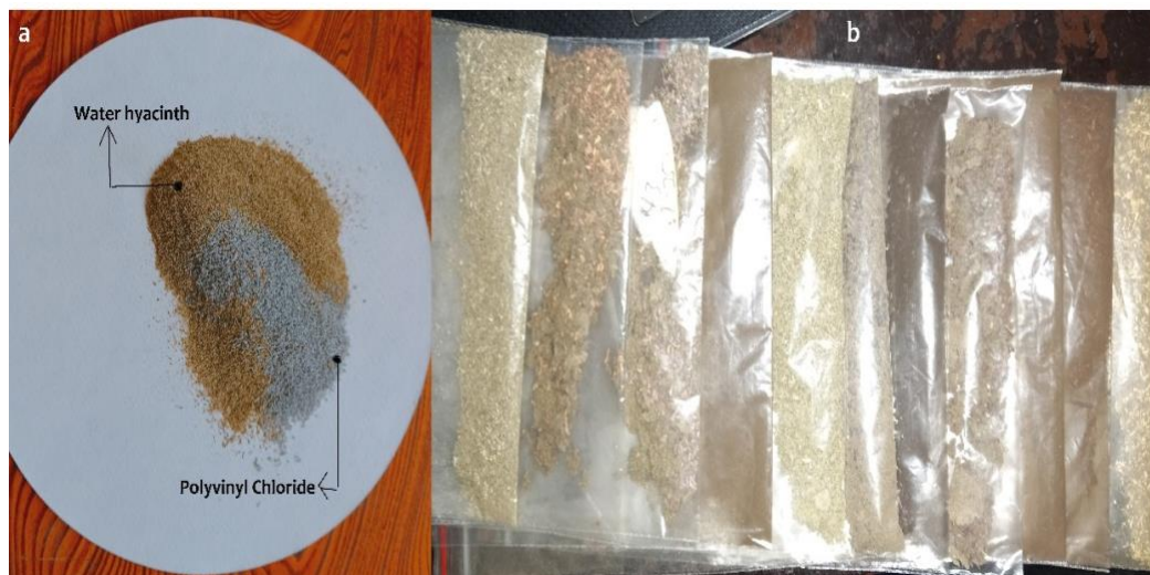
Figure 3.3. (a) The raw PVC and WH feedstock, (b) Samples of Hydrochar produced by Co-HTC of WH and PVC
