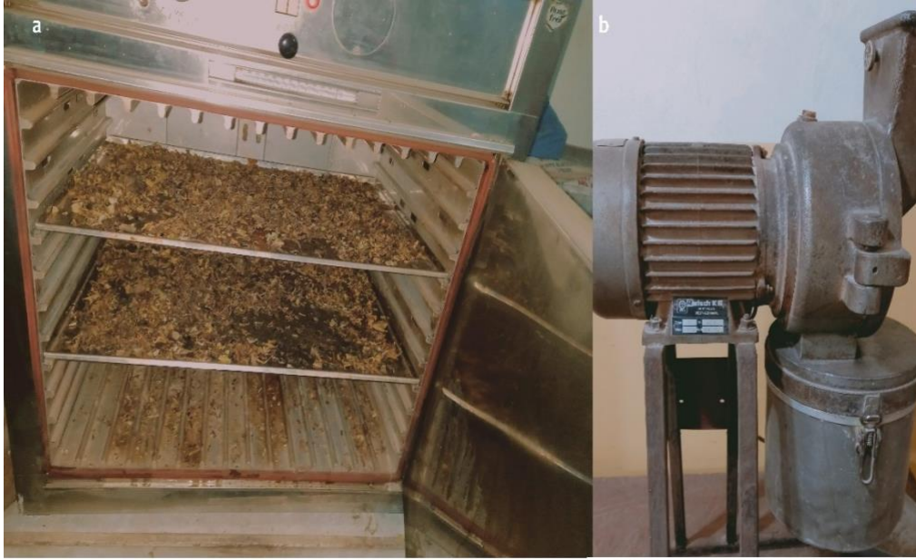
Figure 3.1. (a) Oven dryer used to dry the WH, (b) A hammer mill used to mill the WH.
