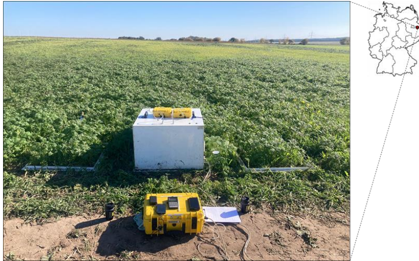
Figure 13: Parallel opaque (Reco) manual closed chamber measurements with a Li-COR 850 IRGA (LI-850, LI-COR, USA) and the developed, low-cost CO 2 and ET flux measurement system.
