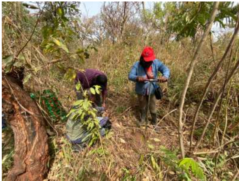
Figure 3.3: Sampling of soil with a core sampler for physicochemical analysis.
