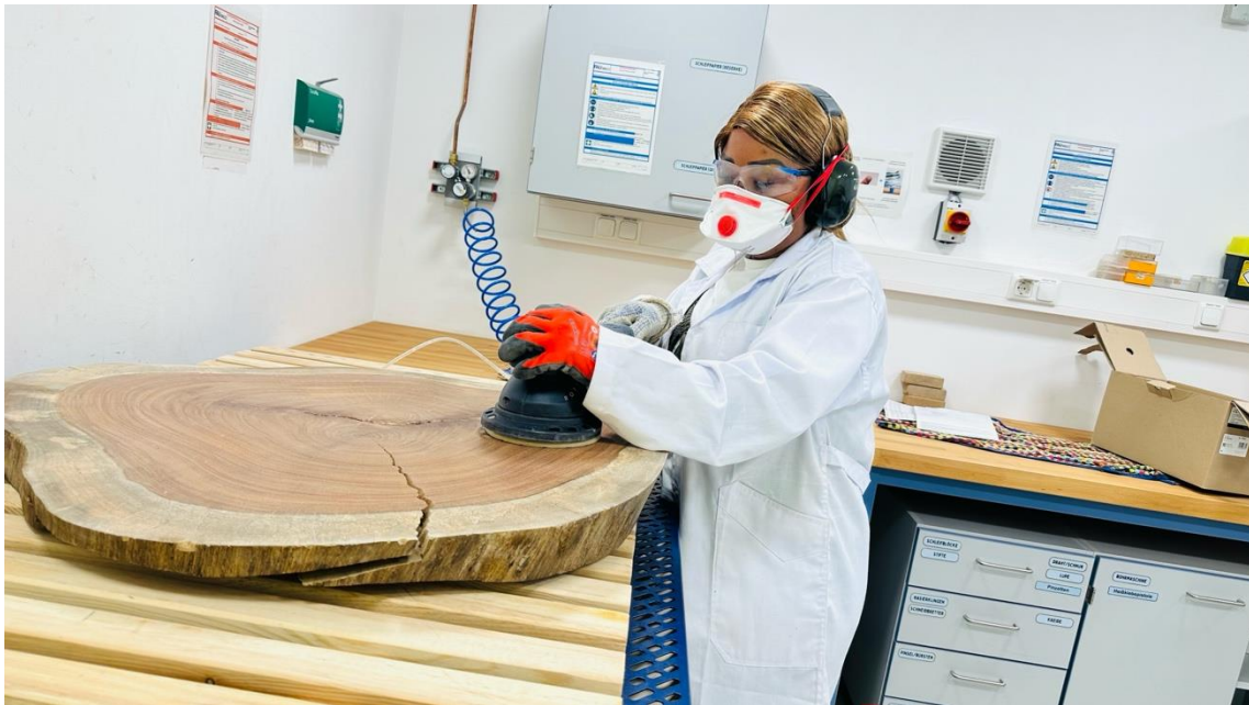
Figure 18: Sanding a disc from an Afzelia africana individual
