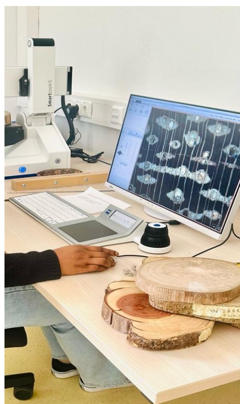
Figure 21: ZEISS Smartzoom 5 automated digital microscope used to visualise the limit of growth rings
