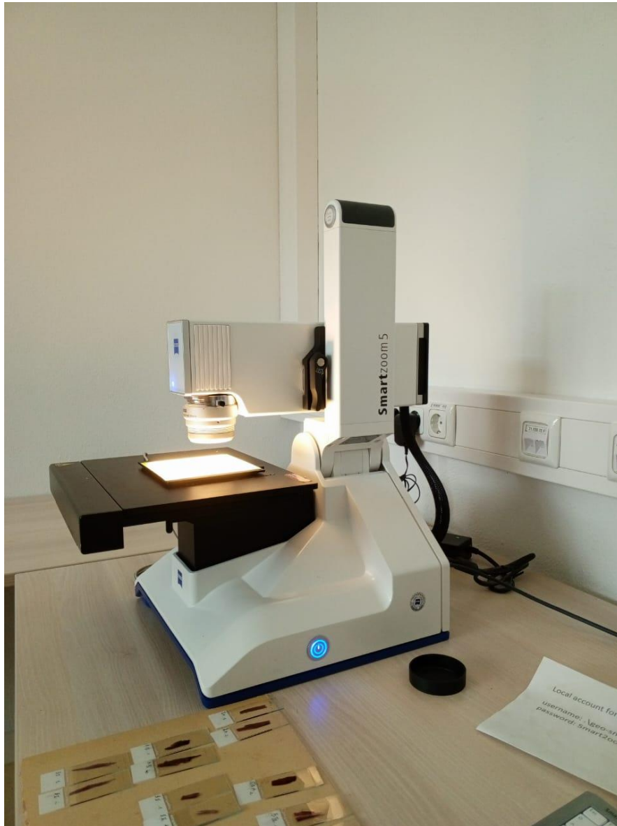
Figure 12: Smart zoom, used to obtain the macroscopic structure from the thin sections of the stem disks.
