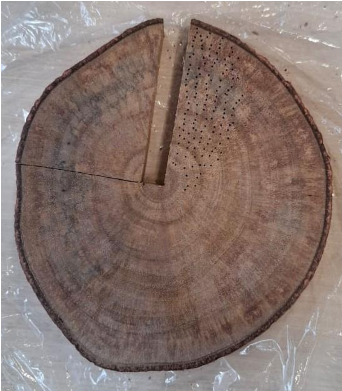
Figure14: Illustration of the collection of wood powders from cashew stem disks
