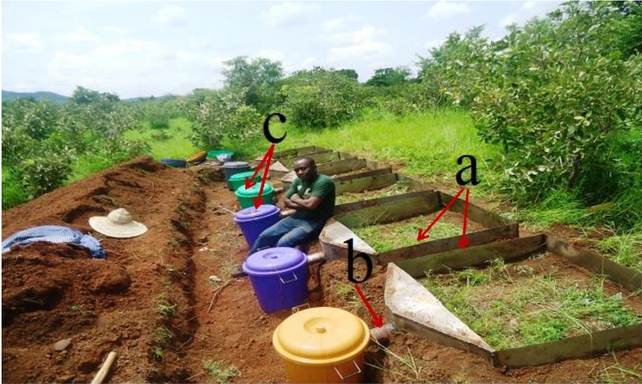
Figure 3.7: Installation of the microplots at the selected site/location, a = microplots, b = outlet, c = collectors (plastic buckets).
