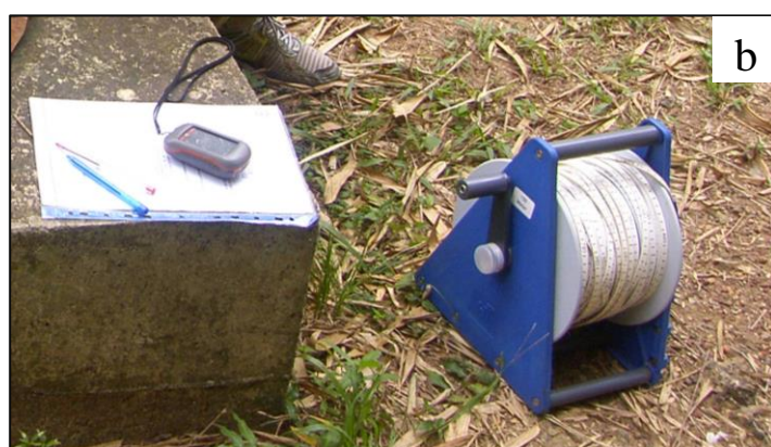
Figure 36: (a) Groundwater level measurement (b): Water level meter and GPS
