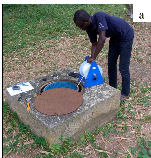
Figure 36: (a) Groundwater level measurement (b): Water level meter and GPS
