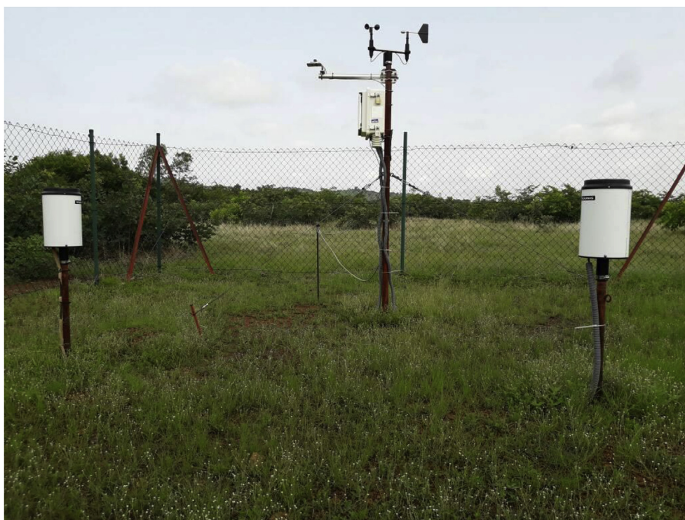
Photo 1. Automatic weather station set-up in Dano catchment with two parallel tipping bucket gauges to depict rainfall uncertainties.
