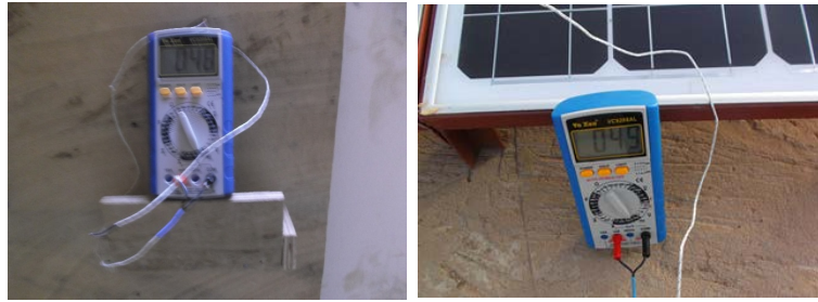
Figure 3. The digital multi-meter with a thermoelectric couple.
