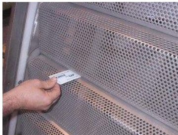
Figure 5: Perforated fine screen (water online)[25]
