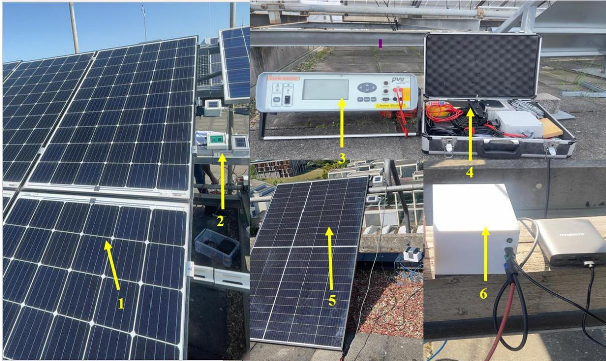
*Figure 4.3. Instruments and solar PV modules during outdoor measurements*
