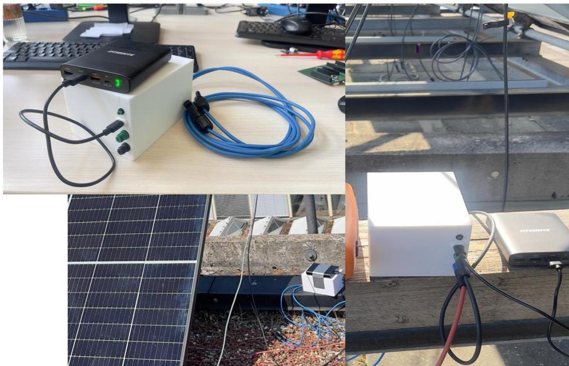
*Figure 4.5. ipv low-cost solar PV Current-Voltage curve tracer*
