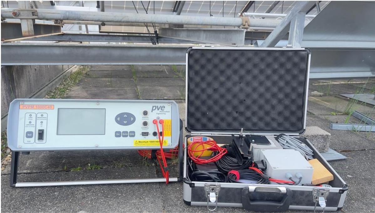
*Figure 4.4. PVP1040C commercial I-V tester along with other hardware and cables*
