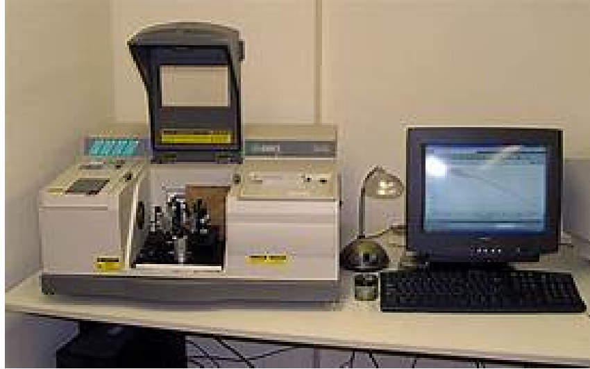
Figure 2: FTIR apparatus for Transmittance Technique
