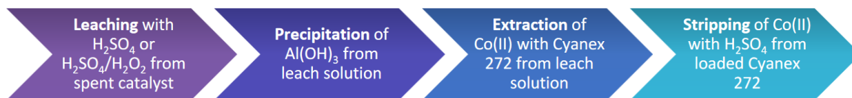
Figure 6: Four-step process for hydrometallurgical recovery of Co(II) from CoMo catalyst of hydrodesulfurization[18].
