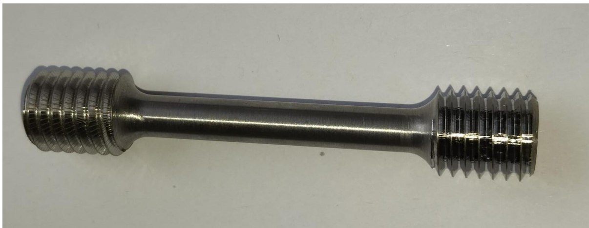
Figure 6: Specimen design as per the ASTM standards.
