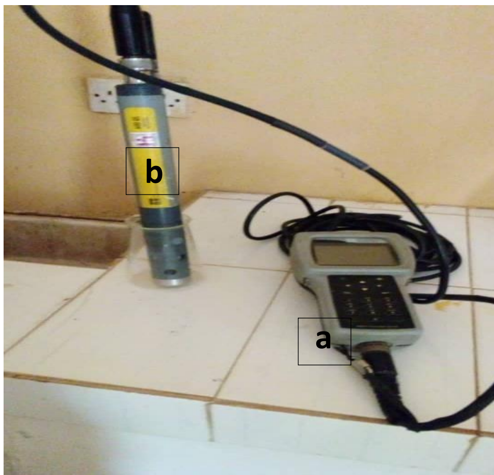
Figure 4: YSI Multimeter equipment (a) and a turbidity column tube (b) for water quality reading, including salinity, dissolved oxygen, temperature; & turbidity respectively.
