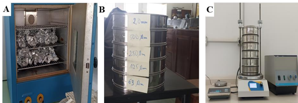
Figure 4: Sediment size post-processing determination: A: drying labelled sediment samples in the oven, (B) a set of sieves on ascending diameter size; C: disposal for sediment sieving (accurate balance, shaker, amperemeter) (credit photo: G. D. Diouf, 2022).
