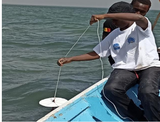
Figure 5: Lowering of Secchi for Secchi depth measurement in the Bétenty elevated bank during high tide (credit photo: G. D. Diouf, 2022).
