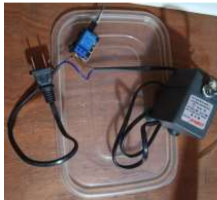
Figure 2.7: Relay and pump Architecture
