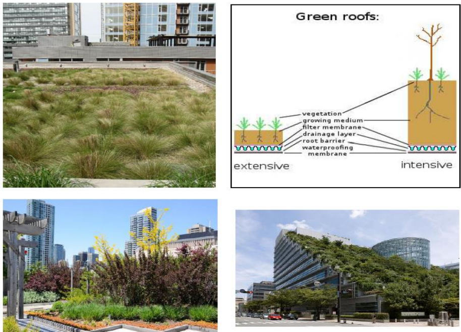
Figure 37: Green roof example and layers
